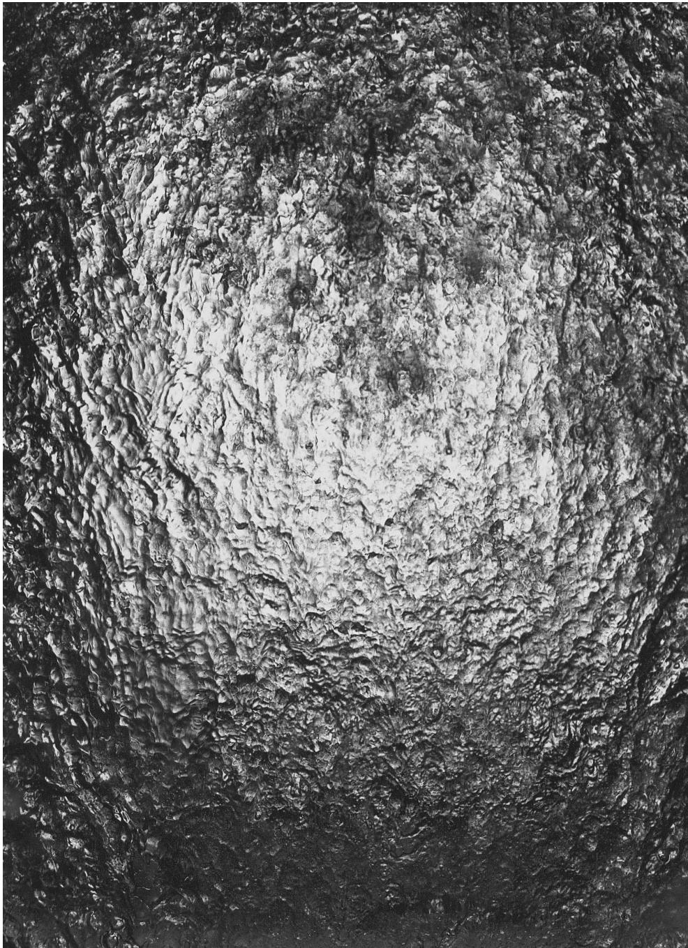
Fig. 8. Photograph of case 2 condition ( j_l = 0.65 m/s, j_g = 20.4 m/s). Magnification = 2.5.
