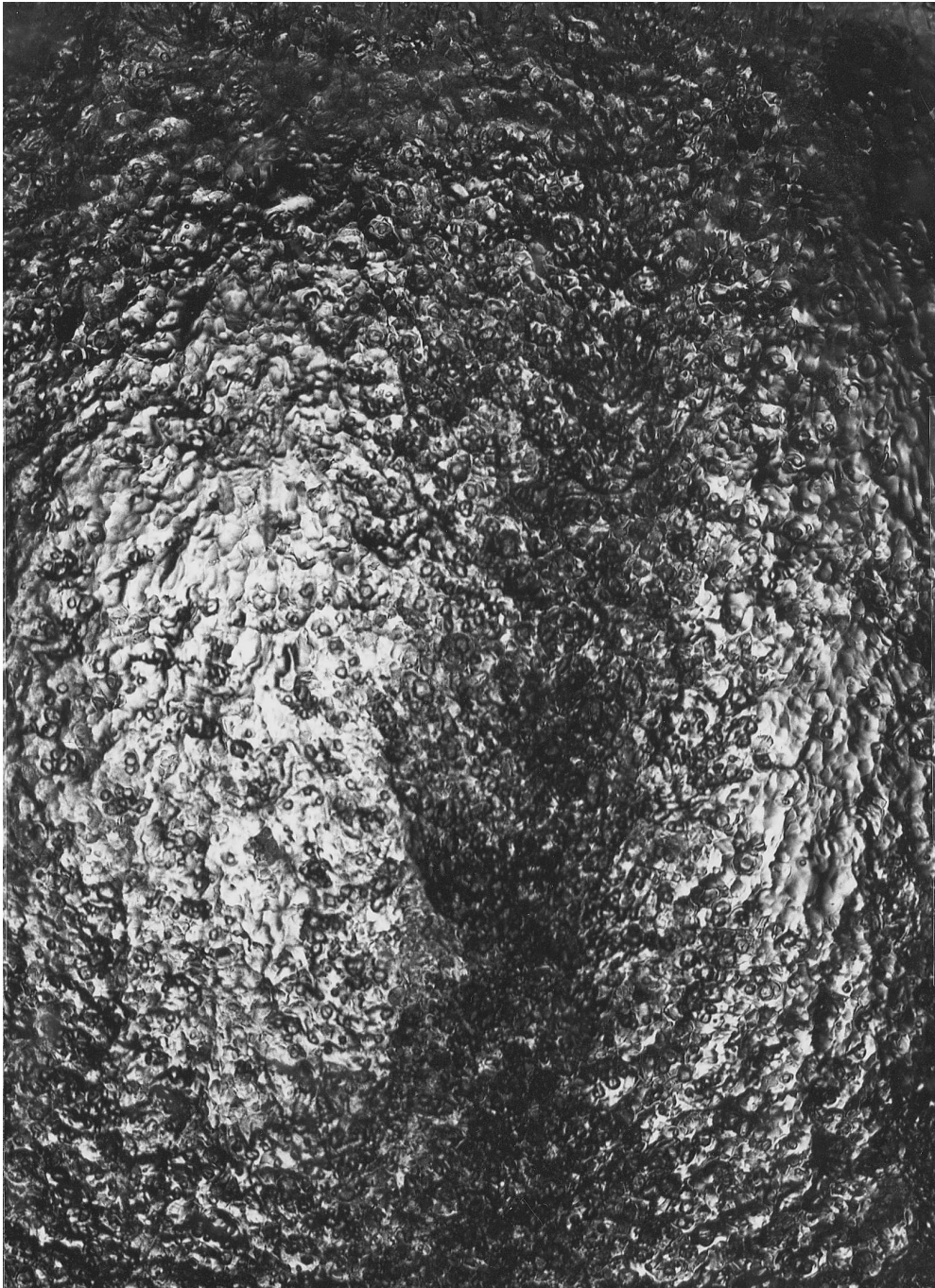
Fig. 7. Photograph of case 1 condition ( j_l = 1.3 m/s, j_g = 12.8 m/s). Magnification = 2.5.
